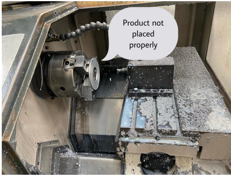
Product Not placed Properly due to which taper cut comes
